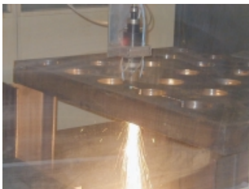
Cutting of a test model of a core support plate
