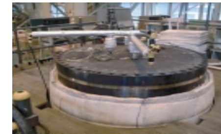
Fire Simulation Test with the same condition as actual cask (simulation of degraded metal gasket) Sealing capability at a fire was confirmed Thermal deformation was evaluated analytically.
