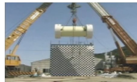
Full Scale Drop Test (simulation of degraded metal gasket) Tight sealing capability when dropped was confirmed. The analytical methodology by non-linear dynamic impact for dynamic behavior of seal boundary was developed.
