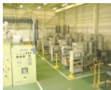
Fatigue Test Facility under the simulated Reactor Water Environment
